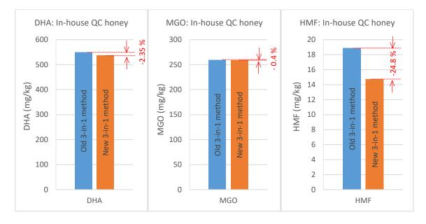
*Figure 2:* Change in results for Hill Laboratories In-house QC honey between the old 3-in-1 method and the new method (average of 30 results each).
