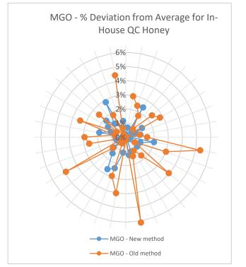
*Figure 4:* Deviation from the average value for MGO in Hill Labs in-house QC honey, run with each batch of customer samples. Orange points were run using the old 3-in-1 method, blue points using the new method. N = 35.
