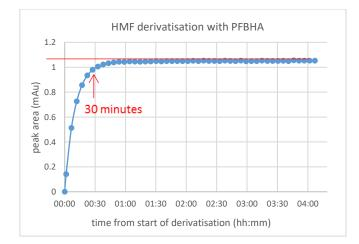
*Figure 1:* Reaction of HMF with PFBHA at 20 °C in acetonitrile/water. The red arrow indicates 30 minutes. Approximate completion of derivatisation is 1 hour 20 minutes.
