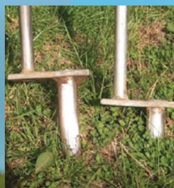
Fig.2 Use a 75mm soil sample auger for collecting soil samples under pasture, or a 150mm auger for crop or horticulture soils.
