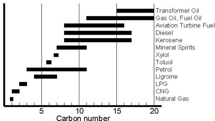
Because hydrocarbon properties depend on the size of the molecules, it is often useful to refer to the number of carbon atoms contained in a hydrocarbon. Volatility (and flammability risk) decreases with increasing size eg C1-C4 are gases, C5-C16 are liquids and higher ones are solids.
