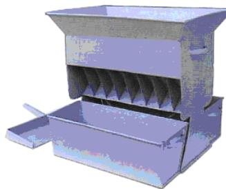
The laboratory uses either of these techniques to reduce the sample size for the DM test. A minimum of 250-300g is advised for most feeds but 500g of maize silage (and other grain-based silages) is required due to the heterogeneous mix of the matrix. Sub-samples should be placed in solid plastic bags with air excluded and sealed well before sending by courier to the laboratory. Samples should be chilled if retained overnight.
