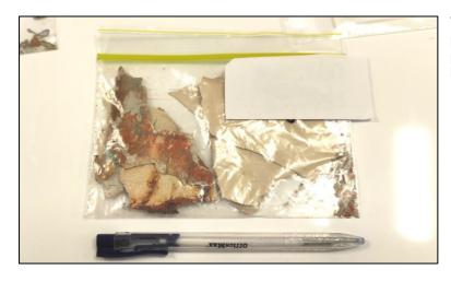
While excessive amounts of paint supplied is preferable to an insufficient amount, it can provide complications for sub-sampling in the laboratory.
