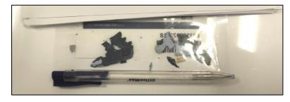
Thick flakes of paint with no inclusion of base substrate (standard pen size for comparison).
