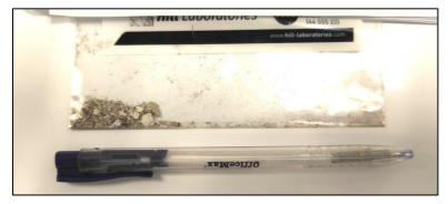
Paint flakes 1mm or less provided with lots of base substrate (non-paint) inclusions.
